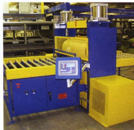
Laminating press with positioned programmed press pressure, speed and gap.
