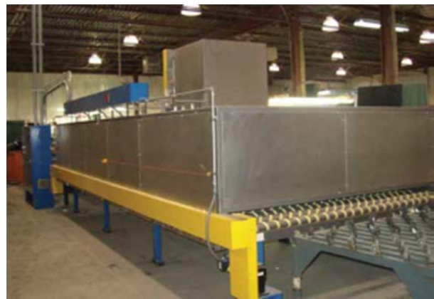
Electric infrared dryer for ceramic and silicone coatings. Photo by Casso-Solar Technologies LLC.
