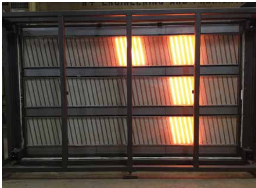
One of the advantages of an infrared heating system is the zoning capabilities. In applications such as paper drying, infrared heater zones can be turned on or off in response to moisture content readings from sensors.
