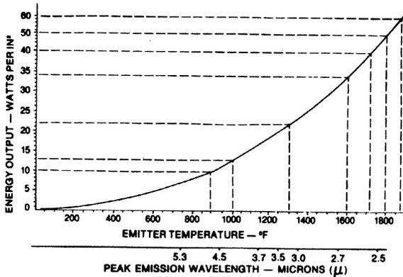
The emission output curve at the left shows emitter temperature versus watt density and the corresponding wavelength emitted for a specific emitter temperature. For example, an emitter temperature of 1300°F would correspond to a peak wavelength of 3.2 microns with a free air watt density of 22 watts per square inch. The key to efficiency is to select the emitter wavelength that best matches the peak absorption of the product to be processed.
