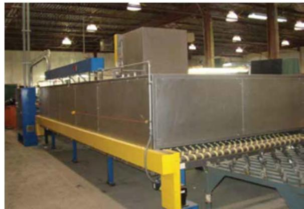
*Electric infrared dryer for ceramic and silicone coatings. Photo by Casso-Solar Technologies LLC.*
